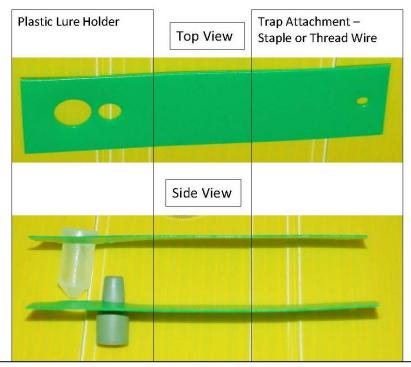
Remember - Lures shouldn't be placed in adhesive or handled with bare hands. Clean disposable gloves should be used for each lure placement; this will prevent cross contamination of pheromones.
